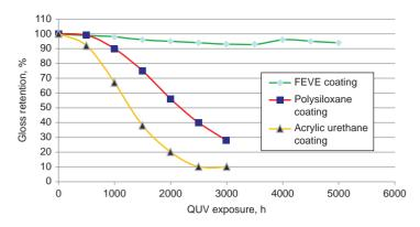
Fig. 4 Exposure of test panels in QUV (Q-Lab Corporation) weatherometer (using UVB-313 light source). FEVE, fluoroethylene vinyl ether
