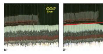
Fig. 8 Micrographs comparing the erosion of (a) fluoroethylene vinyl ether white coating (0 to 1.1 μm, or 0.04 mil, of erosion) and (b) polyurethane white coating (22 to 28 μm, or 0.87 to 1.1 mil, of erosion) after 15 years of exposure. Micrographs property of Asahi Glass Co. Ltd.
