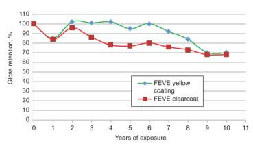
Fig. 7 Exterior exposure of test panels (South Florida exposure site). FEVE, fluoroethylene vinyl ether
